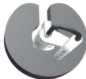
SCARA robots: kidney-shaped envelope with dead space
